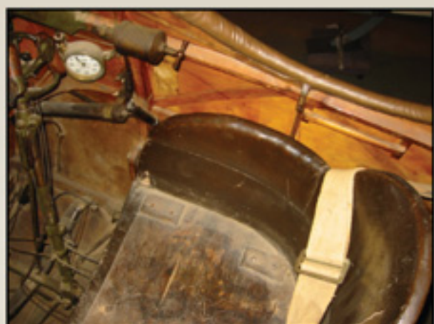
Padded seat and interior longeron detail.
