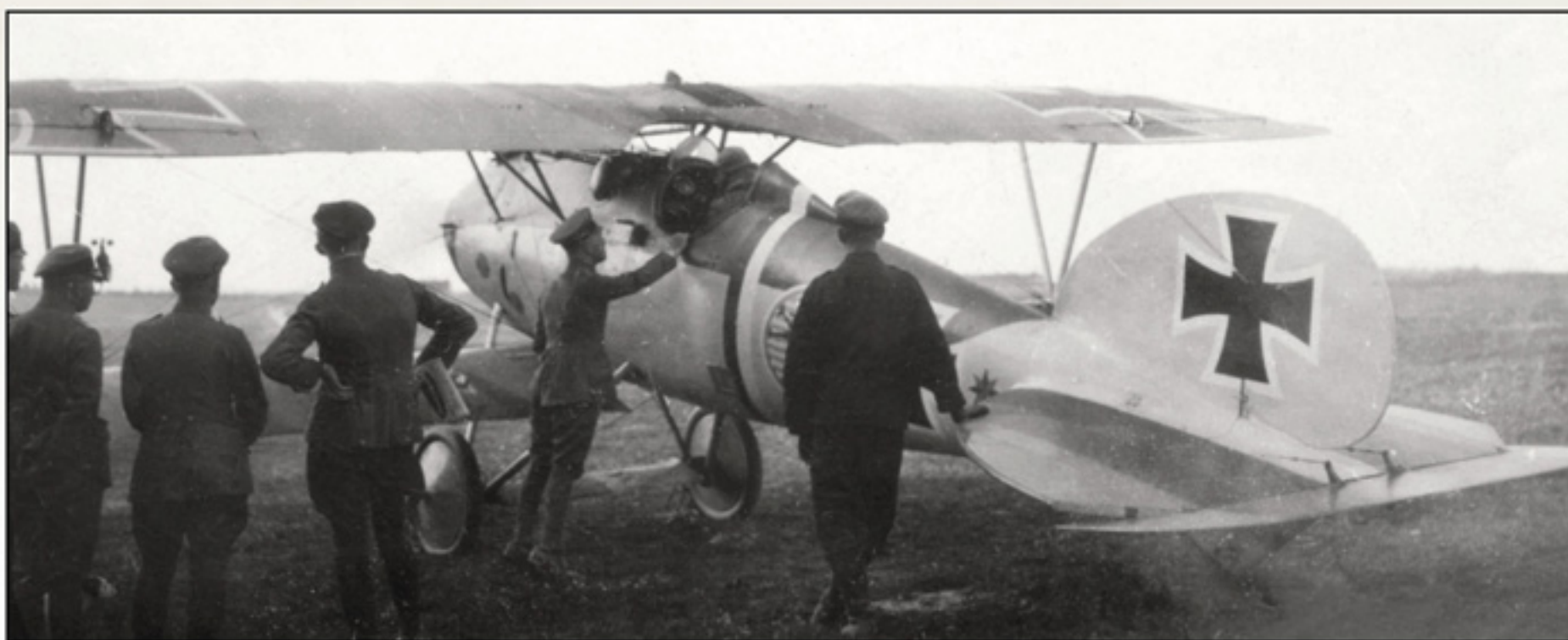
Eduard Ritter von Schleich prepares for take off in D.2034/17. Note the position of the upper wing crosses, strut mounted anemometer, flare rack and that the small scope seen in the following image has not yet been installed. Each half of the undercarriage axle wing upper surfaces appear to have been painted the same mauve and green as the wings. Schleich commanded Jasta 21 from 26 May until 23 October when he transferred to the Bavarian Jasta 32b and became known as 'The Black Knight', with all subsequent aircraft finished overall in black. He survived the Great War with 35 victories and the Pour Le Merite "Blue Max" to his name, flew against the communists in 1919 and joined Lufthansa in 1920. In 1933 he joined the Luftwaffe and commanded various units before becoming General de Flieger in occupied Norway. He died on the 15th of November 1947 in a British POW camp. (Greg VanWyngarden photo)
