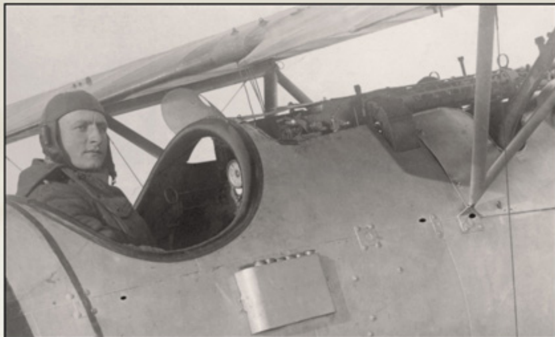
Max Kahlow sitting in the cockpit of his Jasta 34 Albatros D.V. Note the flare rack, ammo chute and windshield with 'peephole' cut out for sighting the guns. Max survived the Great War with 6 victories to his name and went on to become a Lufthansa pilot.
