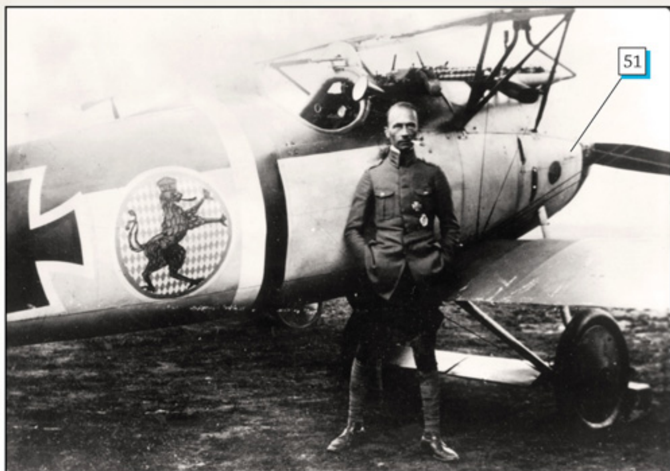
Eduard Ritter von Schleich strikes a famous pose beside the distinctive Bavarian lion personal marking on his Jasta 21 Albatros D.V D.2034/17. Note the small scope protruding through a hole cut in the windshield, the faired in rear view mirror to the right of the cockpit and the very dark (mauve?) appearance of the right wheel cover. The right side engine cowling panels appear to be recent replacements and are possibly unpainted aluminium. (Greg Van Wyngarden photo)
