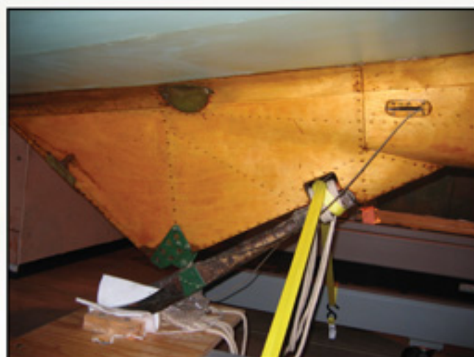
Tailplane detail from D.5390/17. Here we can see the access panels for the rudder control horn, elevator control cable outlet in the fuselage and tailskid brackets. Note the front half of the wooden tailskid is wrapped in linen for strength.
