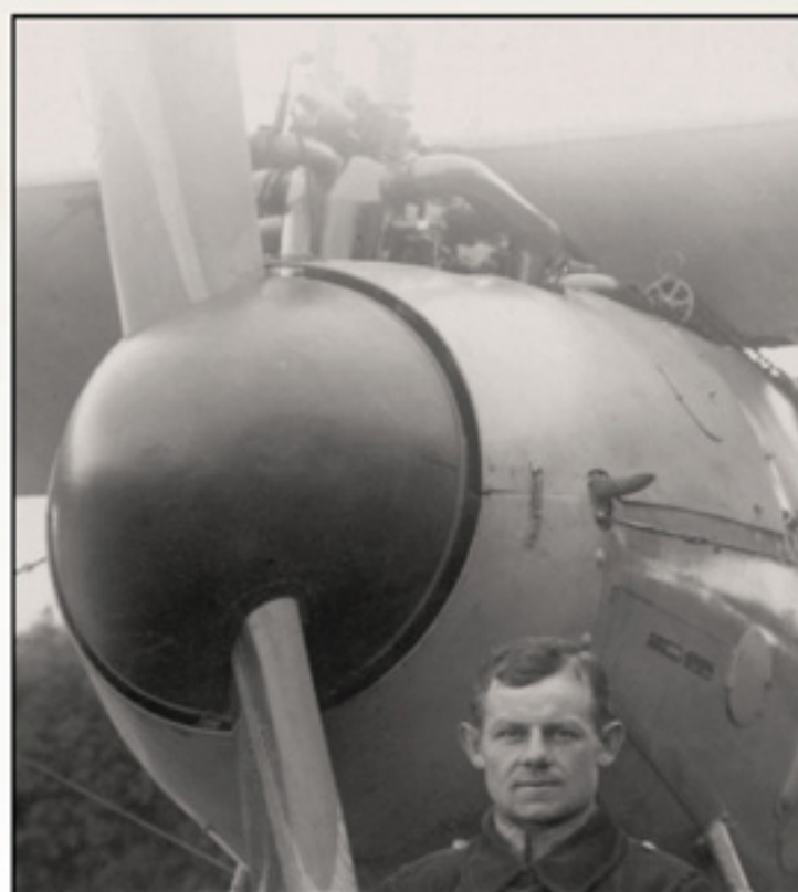
Nose details from Max Müller's Albatros D.V D.1154/17 showing the data plates [51] attached to the left side of the fuselage. Note the foot step and cowling clip just above Max's head.
