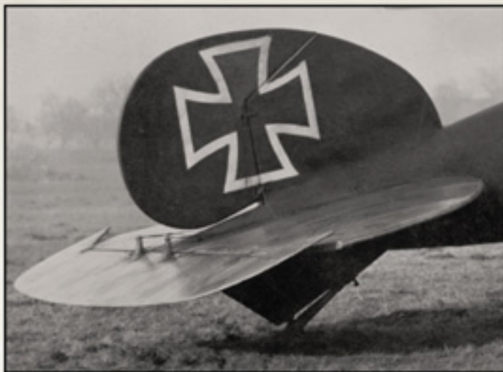
Tailplane detail from Karl Schattauer's Albatros D.V. Note the diamond shaped reinforcing plate on the fuselage in front of the tailplane, a feature not universally applied.
