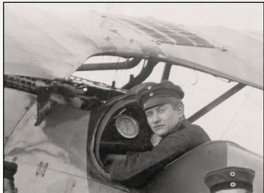
Further fuselage detail of Albatros D.V D.4612. Note that the fairing for the LMG 08/15 empty belt chute has been removed, unusual for the D.V but common for the D.Va, aileron pulley inspection panel and Teeves & Braun radiator.
