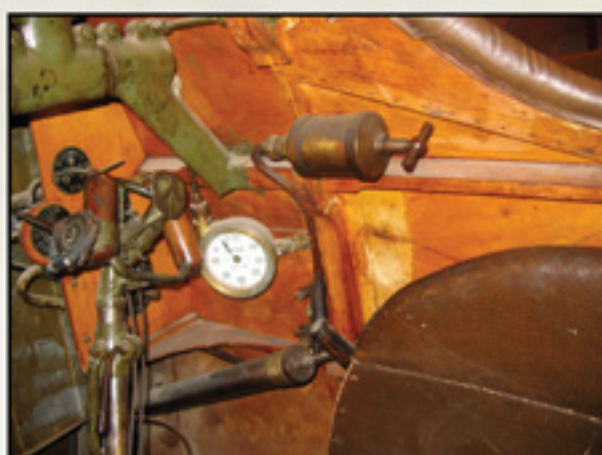
Note the small water pump, larger pump to pressurize the fuel tank and the Maximall fuel gauge.
