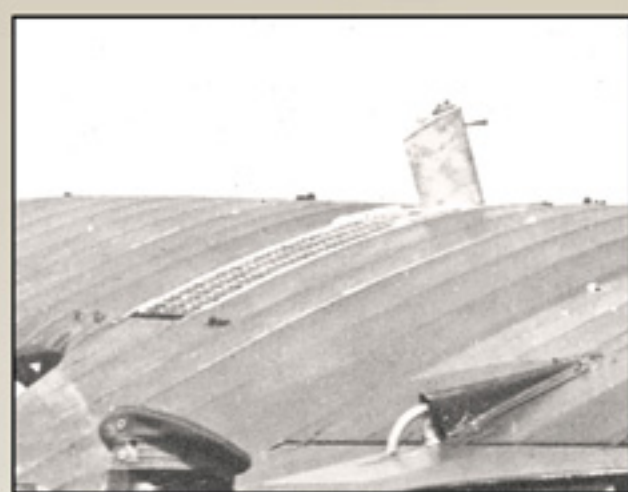
Unpainted aluminium Teves & Braun radiator from Manfred von Richthofen's Albatros D.V. photographed after he was wounded and forced to land during a fight with FE.2ds of 20 Sqn on 6 July 1917.
