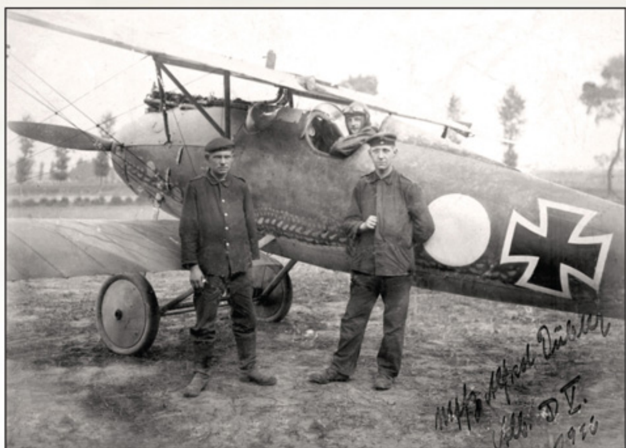
< Karl Haustein poses for a photograph in his well camouflaged Jasta 37 Albatros D.V. Other than the mottled camouflaged paint and the missing 'LO' this aircraft is finished pretty much the same as Ernest Udet's aircraft shown on page 23. Note the small air pump indicating the 160ps Daimler-Mercedes D.III engine, flare rack and safety harness draped over the rear of the cockpit. This aircraft also has additional drag cables to strengthen the wings.
