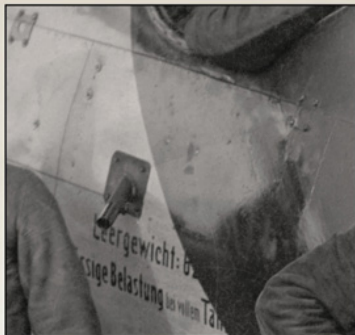
Flare pistol mount from Albert Dietlin's Jasta 41 Albatros D.V D.4612. The positioning of flare pistols and racks was left up to the individual pilots, ensuring a great variety for model makers. Note the weight table partially painted over by Albert's personal marking.
