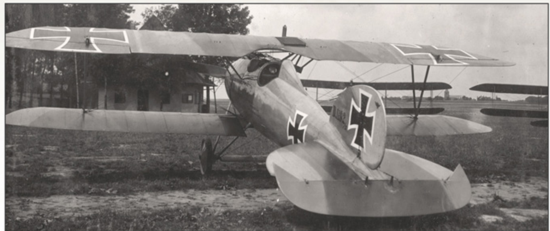
Albatros D.V D.1192. Note the Daimler-Mercedes radiator, headrest, green-mauve-green camouflage and shiny varnished plywood fuselage of this very new D.V.
