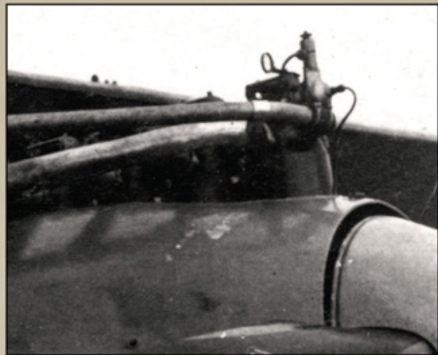
Note the ring sight attached to the top of the engine and the brace from the exhaust to the radiator water pipe in this detail shot of Claus von Waldow's Jasta 15 D.V pictured below.
