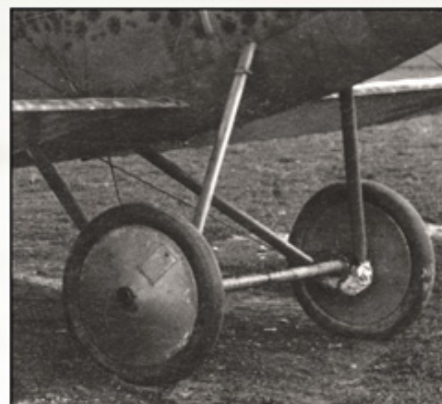
Note the canvas cover protecting the bungee suspension cords on Claus von Waldow's Jasta 15 Albatros D.V.
