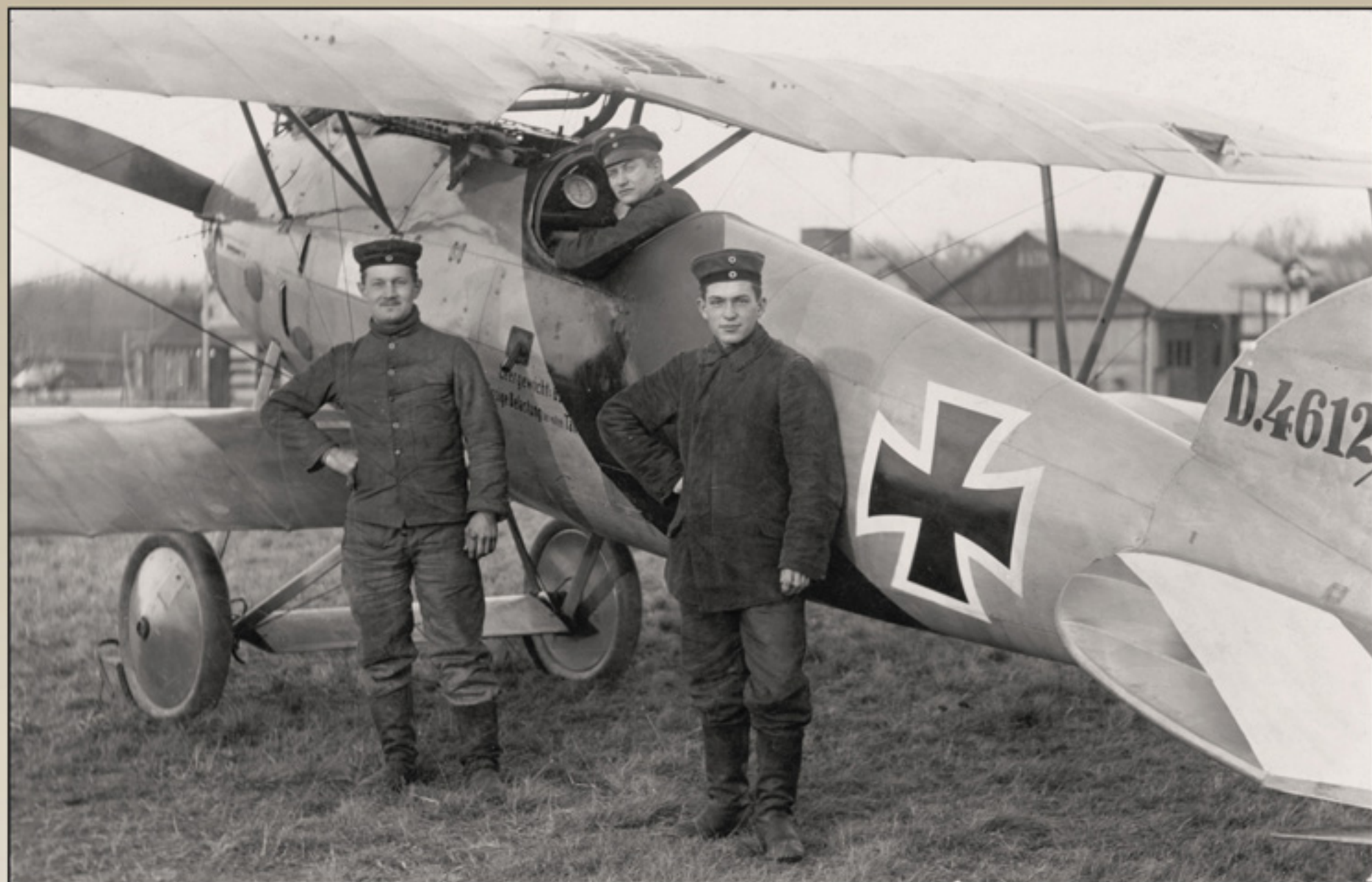
Albert Dietlin's Albatros D.V D.4612/17 in all its glory at Jasta 41. Note the flare pistol, rigging diagram fixed to the left side of the fuselage and missing empty belt chute fairing. Albert Dietlin achieved 9 victories before he was shot down and killed on the 12th of April 1918. He was nearly 28.
