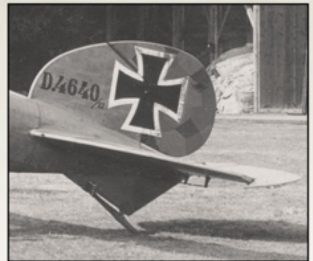
Tailplane detail from Albatros D.V D.4640/17. Note the white paint wearing off the lozenge rudder.
