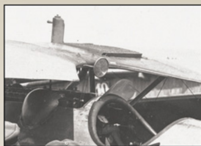
Daimler-Mercedes radiator from Albatros D.V D.2104 of Jasta 19. Note the rear view mirror and that the fuselage shows evidence of the headrest being removed.
