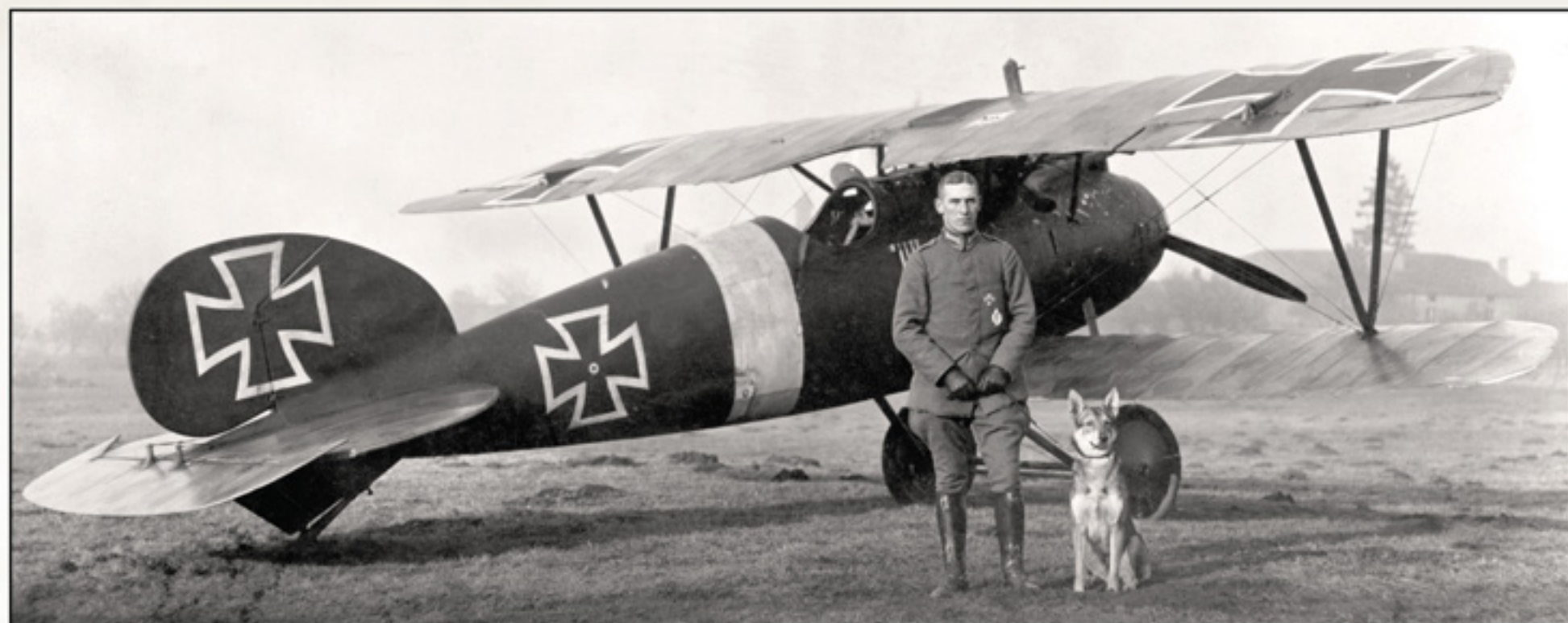
Karl Schattauer poses in front of his Albatros D.V. most likely documenting a recent lucky escape. Two small cockade bullet hole patches have been applied to the fuselage, the most obvious of which is dead center in the middle of the cross, and larger repair patches have been applied to the upper wing. Note the flare rack attached to the right side of the cockpit and Daimler Mercedes radiator. This photo was most likely taken some time after Karl was posted to Jasta 16b on 22 September 1917. This interesting colour scheme will be available from Wingnut Wings shortly.
