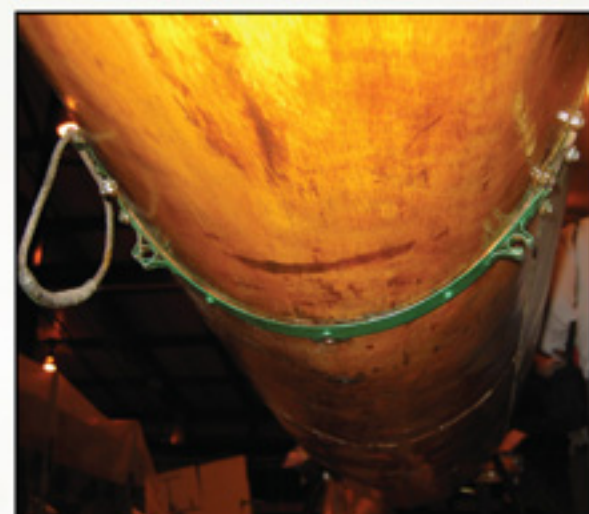
Fuselage lifting handle detail from D.Va D.5390/17 from the Australian War Memorial Museum.
