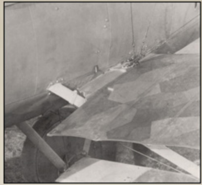
Further detail from Mak Kahlow's Albatros D.V showing how the lower wings attach to the small wooden stubs on the fuselage. Note the rigging attachment points and turnbuckles.
