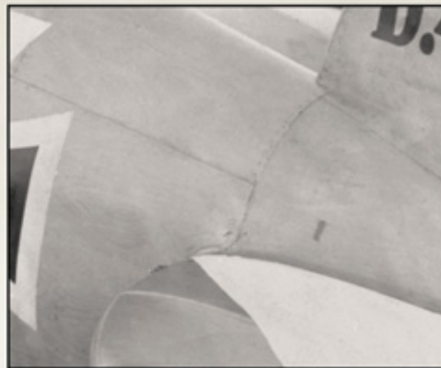
Tailplane detail from Albatros D.V D.4612/17 of Albertt Dietlen. Note the plywood 'grain', panel and nail details.
