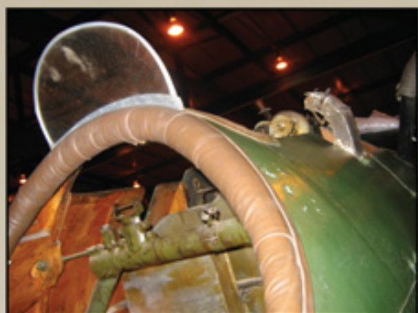
Cockpit padding and LMG 08/15 ammo chute detail.
