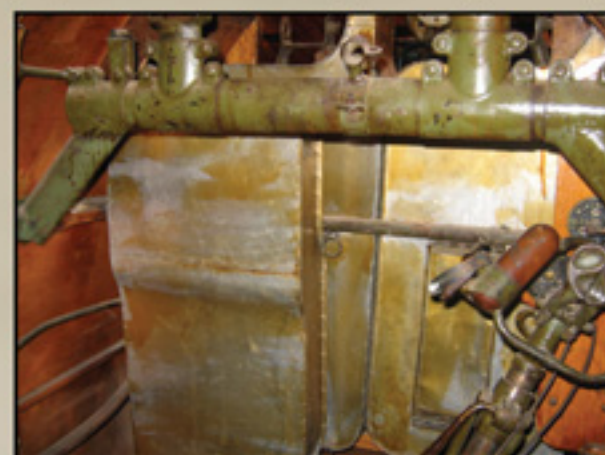
LMG 08/15 mount and empty ammo belt container detail.
