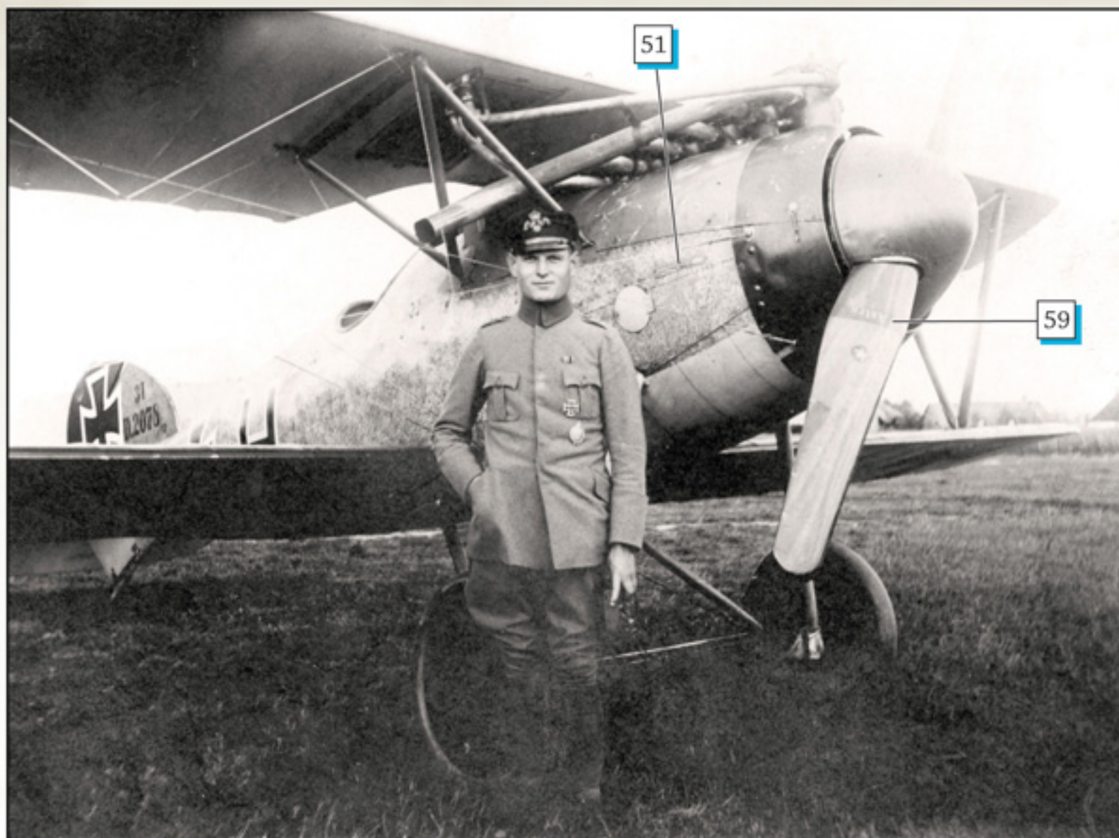
Albatros D.V D.2078/17 of Ottmar Hagenmüller from Marine Field Jasta 1 in late 1917. The orthographic film has caused the chrome yellow of the nose cowl, wheel covers and rudder appear very dark. The fuselage has had olive green camouflage paint dappled on with a sponge at unit level.
