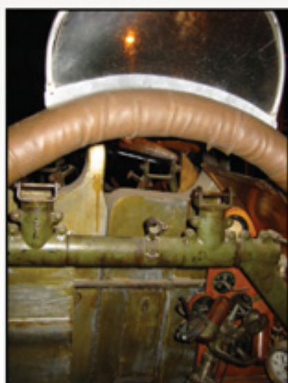
Good view of the LMG 08/15 mount and magazines.
