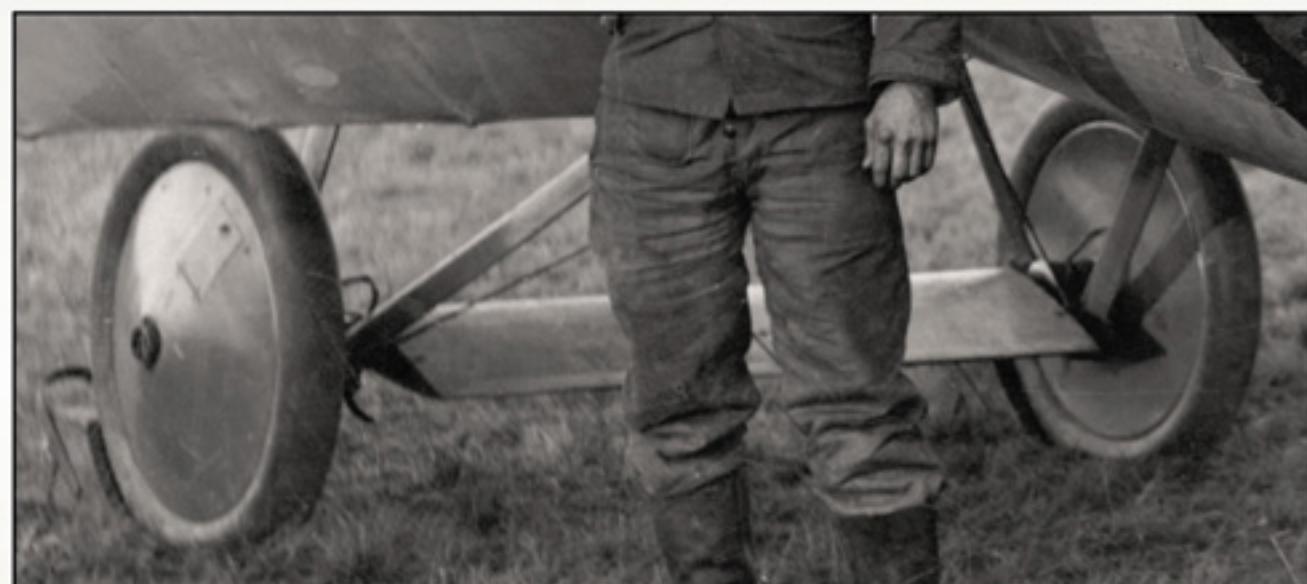
Undercarriage detail from Albatros D.V D.4612. Note the axle retaining cables.
