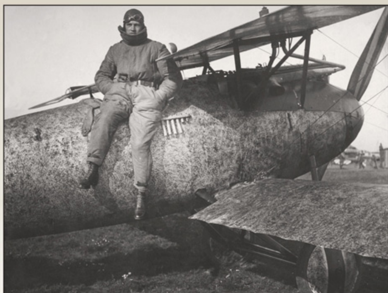
> Alwin Thurm's Jasta 31 Albatros D.V 2058/17 features an interesting reptilian camouflage scheme which has been carried from the fuselage onto the paler green areas of the wings. Note the headrest identifying this as an early production D.V, the Daimler-Mercedes radiator and 160 ps engine. The caption to this photo reads 'Uffz Alfred Dübler Alb D.V 1916 (or 1920)', unfortunately neither date is really appropriate for this scene and no further information about Alfred Dübler has come to light so far.
